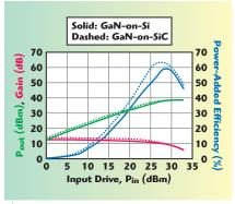
▲ Fig. 7 Representative microwave measurements at 10 GHz for the GaN HEMTs shown in Fig. 6 (solid lines) compared to control samples fabricated on SiC substrates (dashed lines).
