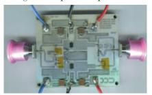
▲ Fig. 1 Symmetric Doherty PA delivering 2 W average in Band 42. The design uses two TQP0103 GaN transistors, each in a 3 × 4 mm plastic QFN package.
