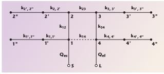
A Fig. 3 Fourth order cross-coupled tri-band BPF topology. Each black node represents a resonator; the lines represent the couplings.
