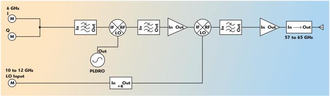
Fig. 1 FEC-15 up-converter.
