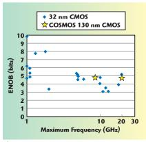
Fig. 5 Effective number of bits (ENOB) vs. maximum frequency for state-of-the-art ADCs compared to the COSMOS ADC. COSMOS performs on par with 32 nm ADCs despite using 130 nm CMOS.
