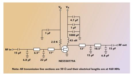
Fig. 5 460 MHz circuit board schematic.
