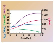
Fig. 6 460 MHz evaluation board - typical performance.
