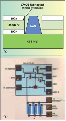
Fig. 6 Cross-sectional schematic of GaN growth on multi-layered Si-based substrate (a). Optical micrograph of Raytheon/MIT's monolithic heterogeneously integrated GaN HEMT + CMOS RF power amplifier circuit (b).
