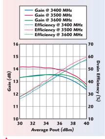
▲ Fig. 2 Symmetric Doherty PA gain and efficiency as a function of output power, using a single carrier, 64 DPCH, 10 dB PAR WCDMA test signal at 3.5 GHz.
