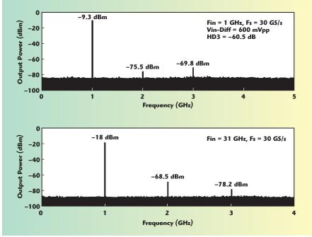
igtriangle Fig.  $8\,$  Differential output spectra for InP BiCMOS T/H amplifier  $^{20}$  (used with permission).
