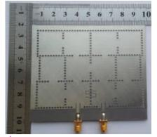
▲ Fig. 6 Photograph of the fabricated triband SIW BPF.
