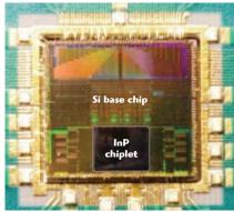
▲ Fig. 4 Micrograph of COSMOS ADC showing InP chiplet and Si CMOS base chip.
