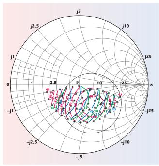
▲ Fig. 4 Load-pull output power, efficiency and gain contours for a QDP3600 carrier amplifier transistor used in an asymmetric, 20 W Doherty amplifier.
