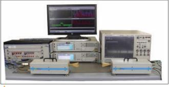
▲ Fig. 3 FEC-15 connected to the Keysight M8190A AWG and the Keysight DSA series oscilloscope with VSA software to analyze the signal.
