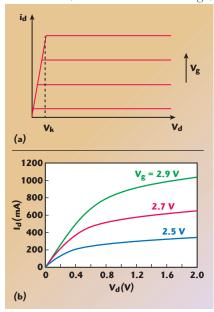
▲ Fig. 1 Idealized transistor I-V curves (a) and I-V curves for NE5550779A FET (b).
