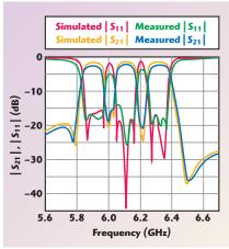
Fig. 7 Comparison of simulated and measured results.
