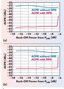
▲ Fig. 3 ACPR vs. output power below P<sub>3dB</sub> for an asymmetric Doherty PA and 10 MHz, 6.5 dB PAR WCDMA signal (a) and 20 MHz, 6.5 dB PAR LTE signal (b).
