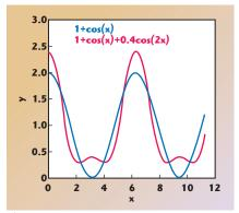
Fig. 3 Flattening effect of the second harmonic component.
