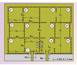
▲ Fig. 4 Tri-band SIW BPF layout.
