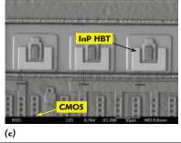
Fig. 3 Heterogeneous integration processes being pursued in the DAHI/COS-MOS thrust: micrometer scale assembly (a) epitaxial layer printing (b) and monolithic epitaxial growth using a multi-layered lattice-engineered substrate (c).
