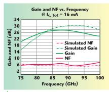
▲ Fig. 9 Gain and noise figure versus frequency for InP BiCMOS W-Band LNA<sup>21</sup> (used with permission).
