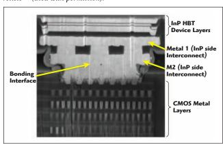
▲ Fig. 11 SEM FIB cross section of DAHI Foundry Technology heterogeneous interconnect (HIC)<sup>23</sup> (used with permission).
