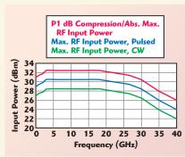
▲ Fig. 1 PE42524 switch power handling capability at 25°C and 85°C ambient.
