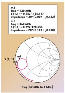
Fig. 8 Load impedance simulation of the standard evaluation circuit.
