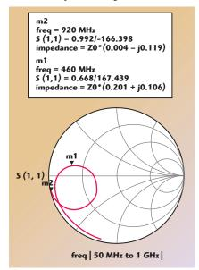
Fig. 9 Load impedance simulation after tuning for the Class J mode.
