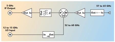
Fig. 2 FEC-15 down-converter.
