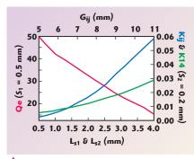
▲ Fig. 5 Extracted external quality factor and coupling vs. physical parameters.
