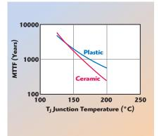
▲ Fig. 1 MTTF comparison of plastic over-molded and ceramic air cavity packaged transistors
