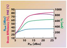
Fig. 10 Actual performance with the Class I matching network.
