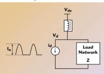
ightharpoonup Fig. 2 Equivalent circuit and half-sine waveform of  $i_d$ .
